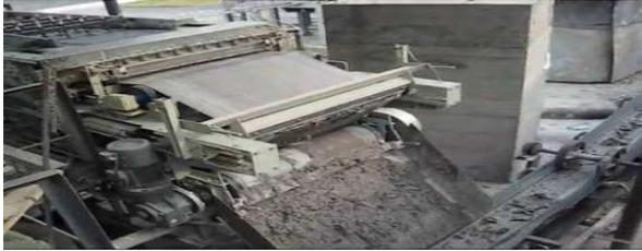
The belt filter is used for solid/liquid separation processes.
